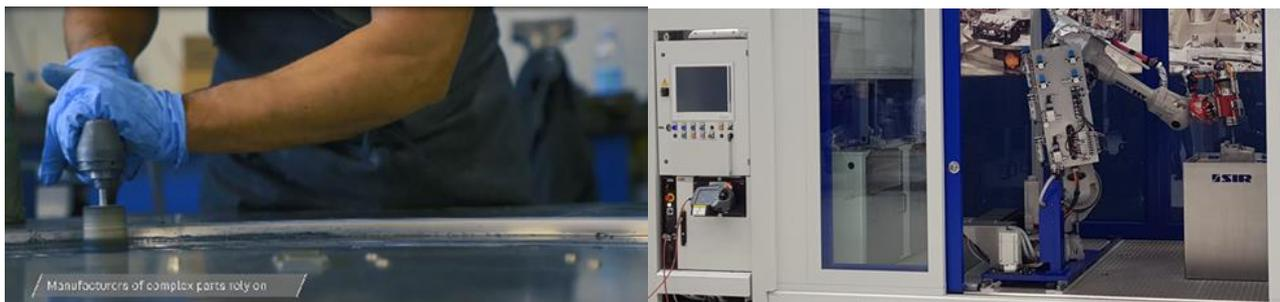
*Left panel shows today's manual polishing. Right panel shows tomorrow's automatic polishing. The QISAB systems are essential in order to perform automatic polishing, including direct process feedback and AI/human decision making.*
